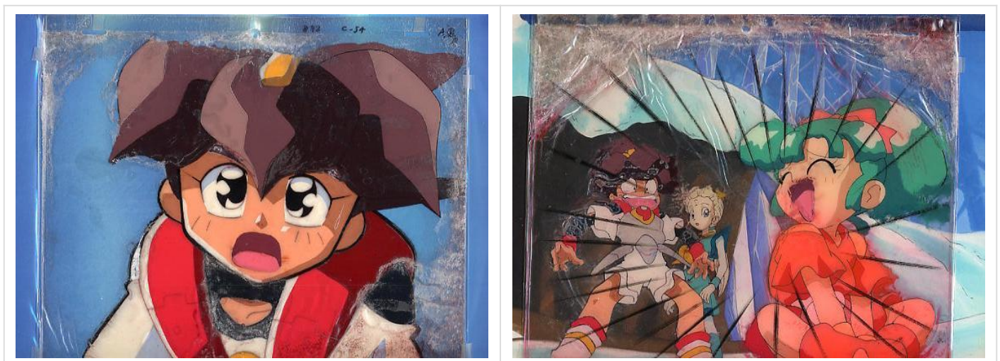
Examples of cel warping/rippling, indicative of vinegar syndrome.
